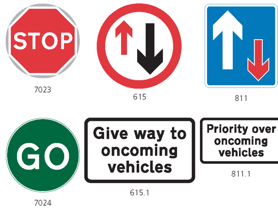
Figure 3.5: Manually Operated Stop/Go Signs and Priority Signs.
